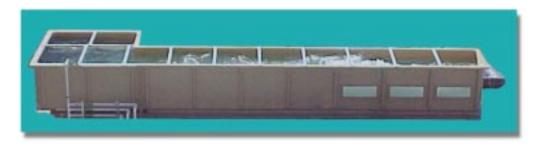
High-velocity test flume showing flow from right to left. The flume measured 9 m long x 1.2 m wide x 1.2 m deep. An electric pump capable of producing exit velocities in excess of 20 m/s was used to produce a consistent shear environment. Viewing windows at the sides and bottom were inserted to facilitate video recording.
