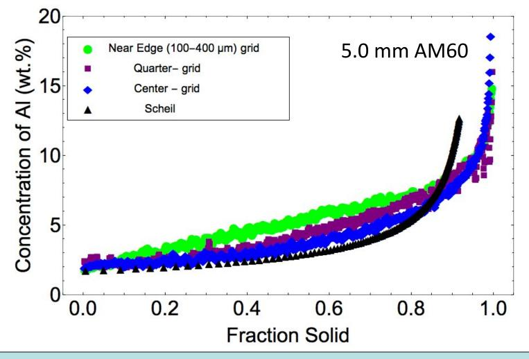
Microsegregation deviates from Scheil as you move towards the edge of the casting
