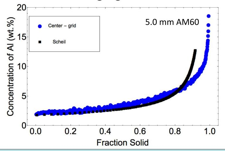
EPMA microsegregation profile at the center of the castings is close to Scheil up to a high solid fraction
