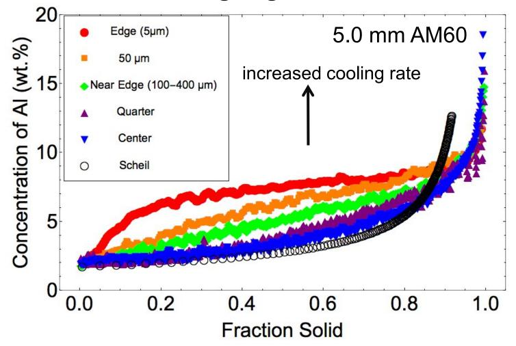
Solute trapping increases near the edge of the plate where cooling rate is the highest
