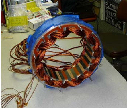
Flux-Switching Dy-Free PM Motor Prototype
