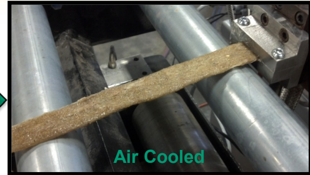
Die redesigned for minimum shear producing compounded Tape Form
