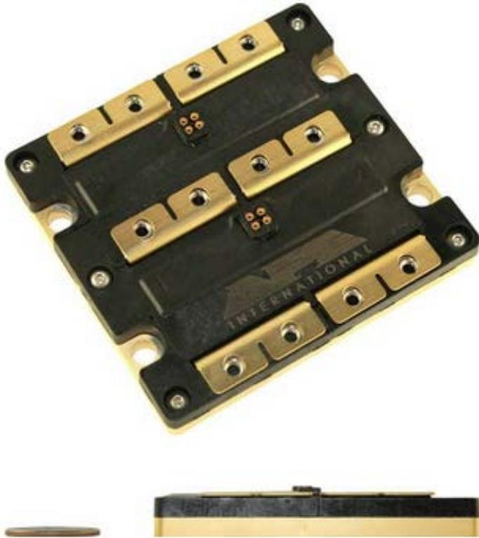
*APEI, Inc. HT-2000 WBG Device-Neutral Power Module. 1200 V and up to 1000 A half-bridge in a 3" × 3.2" × 0.5" package. U.S. Quarter for scale.*
