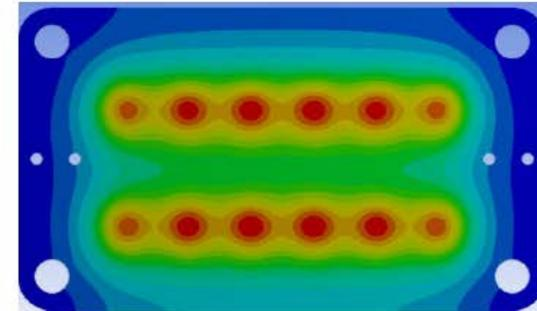
Temperature profile of bottom of base plate
