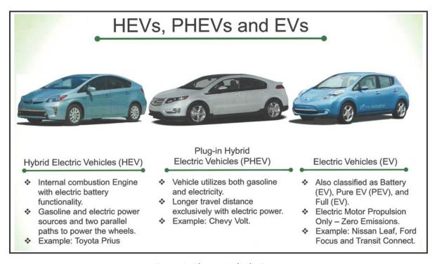
Figure 2: Electric Vehicle Types
