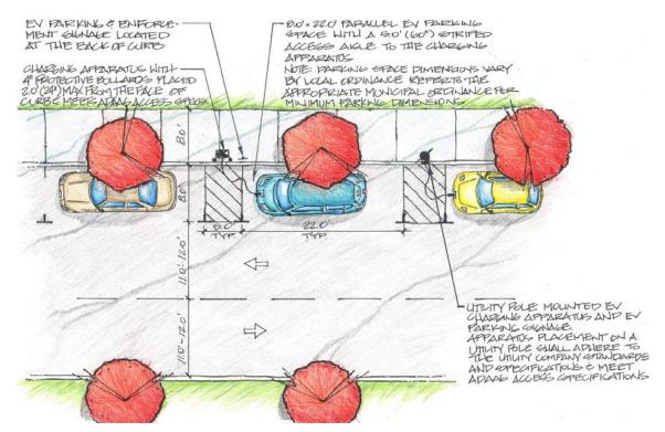
Figure 13: Example Layout for On-Street Parallel Parking
