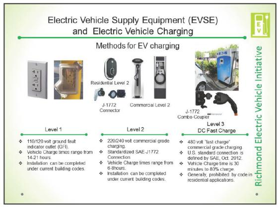
Figure 3: Electric Vehicle Supply Equipment
