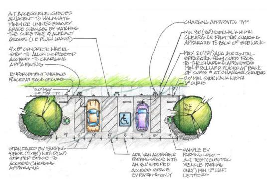
Figure 11: Example of 90-Degree EV Parking Adjacent to Sidewalk
