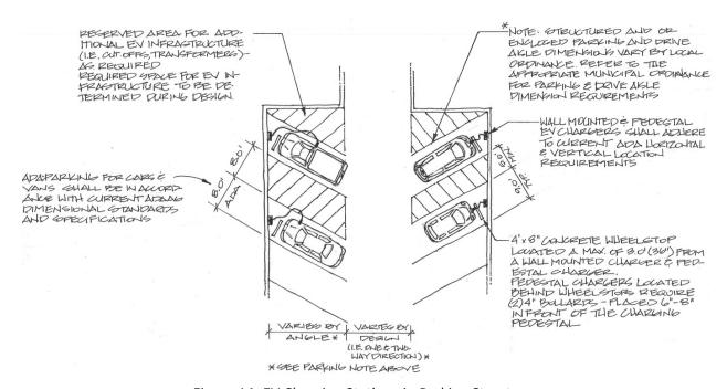
Figure 14: EV Charging Stations in Parking Structures
