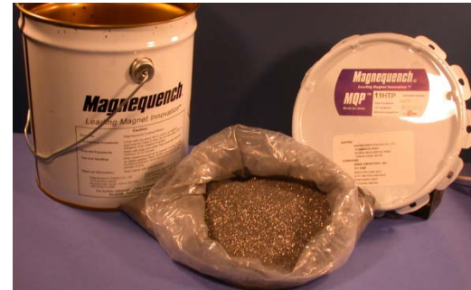
Portion of 100kg batch of 11HTP Ames alloy flake.
