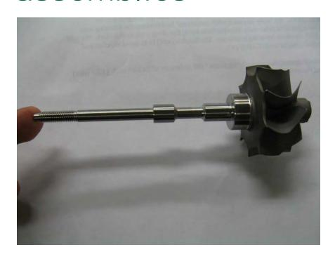
Honeywell supplied wheel/shaft components from gasoline turbocharger products
