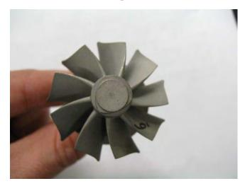
HTML User-Center at ORNL will use neutron-scattering to measure residual stresses in the weld-joint between Ni-based superalloy wheel and steel shaft
