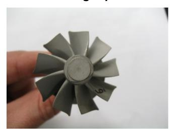
HTML User-Center at ORNL used neutron-scattering to measure residual stresses in the weld-joint between Ni-based superalloy wheel and steel shaft
