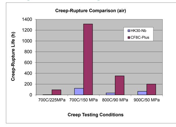
Creep-Rupture Testing of Cast CF8C-Plus stainless steel and HK30-Nb stainless alloy at ORNL
