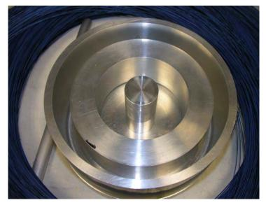
Designed and fabricated fixture for building a DC+(high frequency) excitation core Fabricating an experimental excitation core
