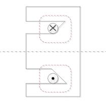
Cross sectional view of motor excitation core
