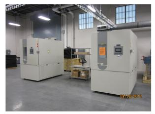
Figure II - 113: View of mid-size thermal temperature chambers delivered in FY12.
