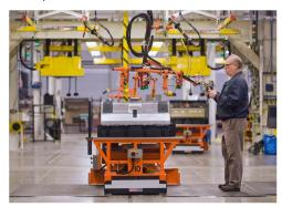
Figure II - 48: Battery Pack Lift Assist.
