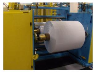
Figure II - 55: Celgard Fully-formed flat sheet membrane from new equipment.
