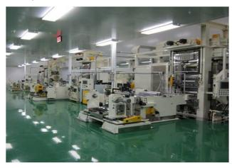
Figure II - 30: The roll press equipment for the electrode process.
