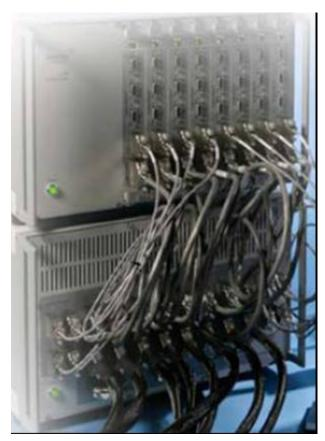
Figure II - 97: Solartron (Ametek) eight channel electrochemical test station and impedance analyzer.
