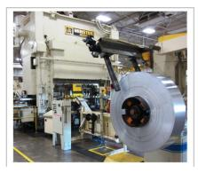
Figure II - 86: Equipment – Battery Can Stamping Press (HTTM LLC, H&T, Trans-Matic).
