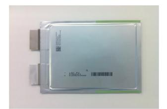
Figure II - 34: The Li-ion battery cell produced during the equipment validation process.
