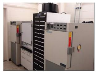
Figure II - 94: Maccor Series 4000 Automated Test System for testing and formation of prototype cells with environmental chambers and ovens.
