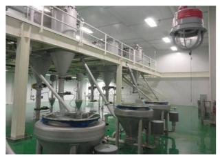
Figure II - 29: The bag filters on the  $4^{th}$  floor of the mixing tower of the electrode process.
