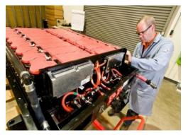
Figure II - 9: Complete battery packs and systems are assembled domestically prior to being sent to the customer.
