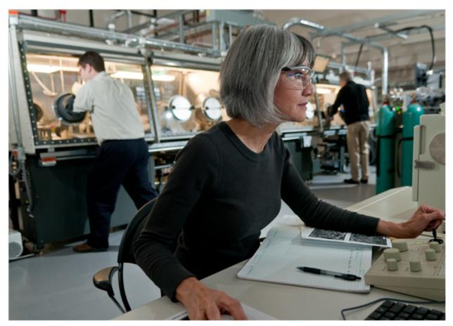
Figure II - 108: Argonne scientist Nancy Dietz Rago analyzes results in the Post-Test Facility. After a battery sample is characterized in the large glove box, it is transferred without exposure to air to the scanning-electron microscope for detailed, microstructural characterization.
