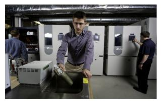
Figure II - 122: Environmental chambers and isothermal bath for battery cell and pack testing.
