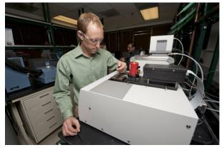
Figure II - 121: Laser Flash Thermal Conductivity Meter for thin battery electrodes.
