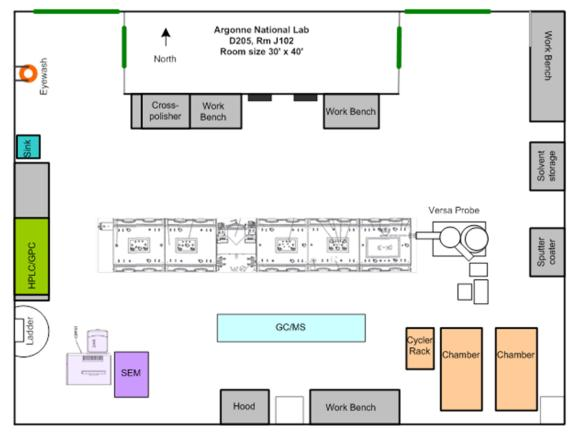
Figure II - 107: Overall design of the post-test facility. The large, open area at the top of the figure is not part of the post-test facility. The VersaProbe X-ray photoelectron spectrometer (XPS) was purchased with funds from the US Department of Defense.
