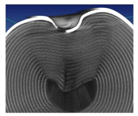
Figure II - 125: CT image of an 18650 lithium-ion showing the mechanical abuse failure point in the electrode roll.
