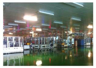
Figure II - 32: The end of line inspection equipment for the formation process.
