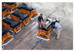
Figure II - 49: Battery Pack Assembly on Automated Guided Carts.
