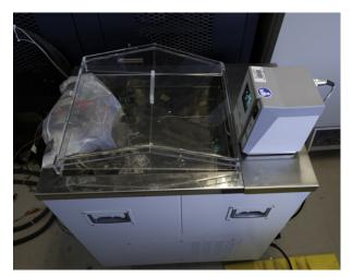
Figure II - 120: Isothermal Bath with battery under test.
