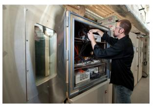
Figure II - 123: Life cycle testing of batteries for secondary use applications.
