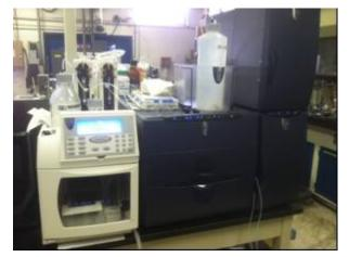
Figure II - 75: Ion Chromatograph (Novolyte).
