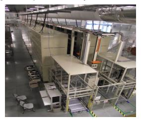
Figure II - 38: Cell Formation Equipment - Mt. Comfort.
