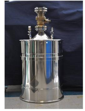
Figure II - 69: Special container for shipping finished product.
