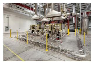
Figure II - 73: EnerG2 Pyrolysis Kilns.
