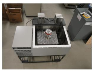
Figure II - 118: NREL Designed and Fabricated Cell Calorimeter in Fluke Isothermal Bath.
