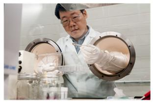
Figure II - 106: Glovebox for Coin Cell Fabrication (ANL).
