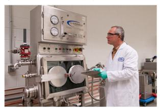
Figure II - 105: Filter-Washer-Dryer Unit (ANL).
