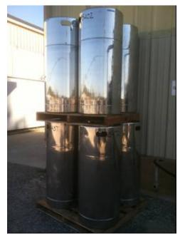
Figure II - 74: Several examples of the 400 215-L Electrolytes shipping vessels purchased in 2010 (Novolyte).
