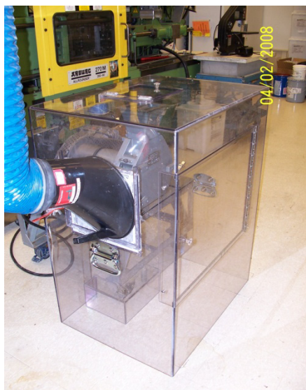
Figure 20. Wiley mill with polycarbonate containment enclosure.
