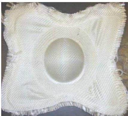
Figure 2. Formed hemisphere using the thermo-stamping process.
