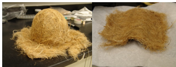
Figure 21. Preform hat section and curved pieces.
