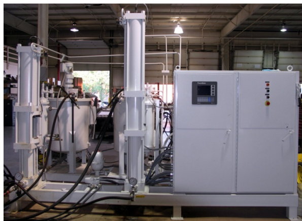
Figure 2. Urethane injection system capable of 110 pounds (lb)/minute and 33 lb shot sizes.
