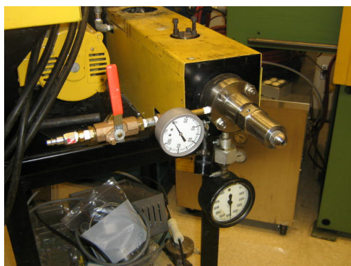
Figure 18. Current extruder apparatus with adapted tip. This work continues into FY 2009; results will be reported upon determination of the process viability.
