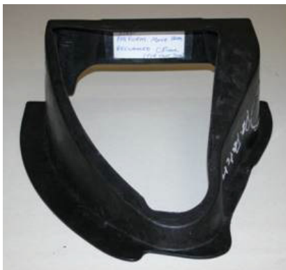
Figure 1. Corvette wheelhouse lower support demonstration part molded at MFG using a carbon fiber preform made by the 3-DEP process.
