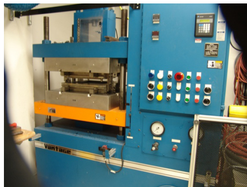
Figure 22. PNNL SMC plaque tool (in press), producing kenaf-reinforced panel.
