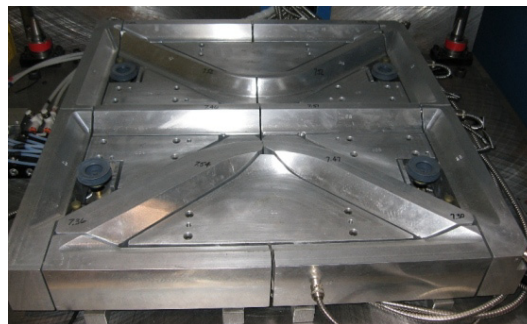
Figure 2: The bonding fixture in the “full nest” configuration.
