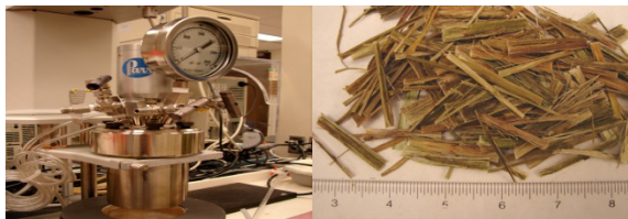
Figure 10. Parr high-pressure reaction system (left) and 1.5-in. decorticated kenaf fibers.
