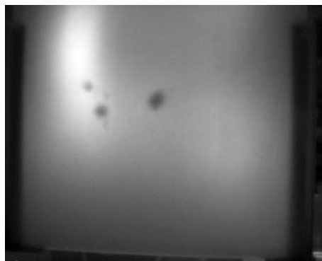
Figure 16. Infrared thermal wave image showing three blisters present in an SMC test panel.
