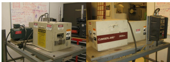
Figure 8. Pelletizer used to chop fiber into specified lengths.
