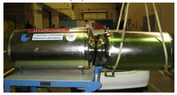
Figure 1. Generation 2 cryo-compressed hydrogen storage tank prototype (left). Generation 3 cryo-compressed hydrogen storage tank prototype (right).
