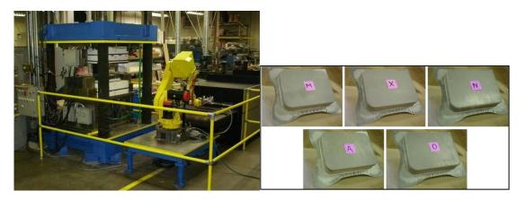
Figure 1. Warm forming cell capable of five jobs per minute and pans stamped at 350°C from five different magnesium alloys.
