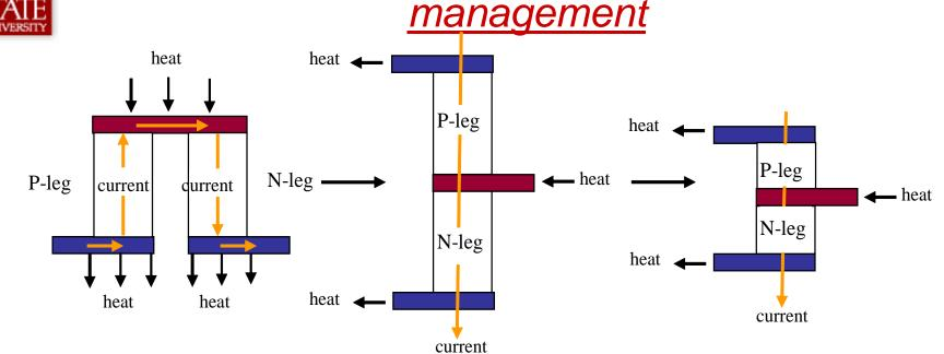
Heat / electrical current in cross-flow geometry
