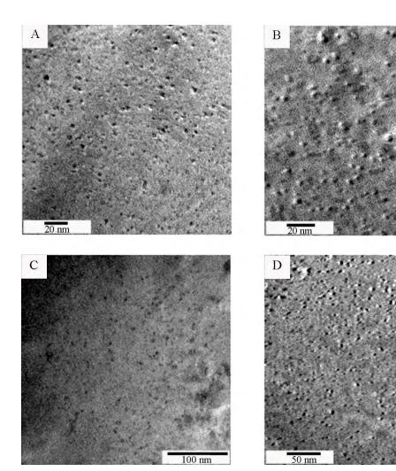
Dispersed nanoparticles in samples of Sb-doped PbTe: (A)PbTe-Sb(2%) (B)PbTe-Sb(4%) (C) PbTe-Sb(8%) and (D) PbTe-Sb(16%).
