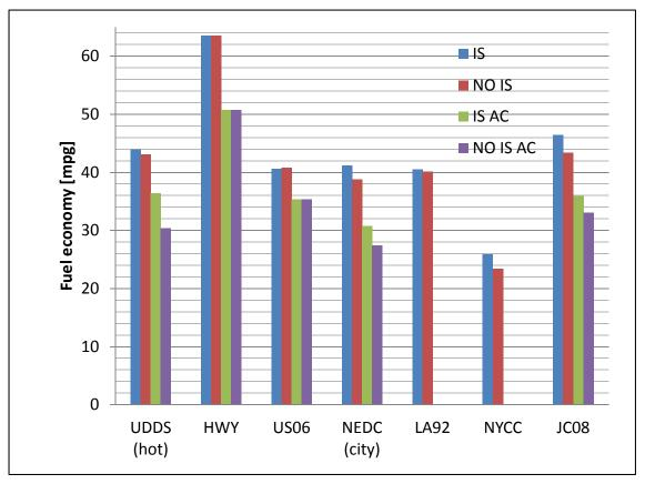
Figure 3. Volkswagen dynamometer test results comparison.
