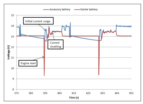
Figure 6. Mazda vehicle battery usage during engine starts.
