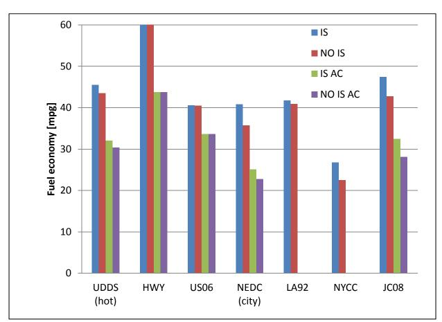
Figure 1. Smart vehicle dynamometer test results comparison.
