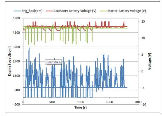
Figure 5. Mazda vehicle New York City Cycle battery voltages and engine speed versus time.
