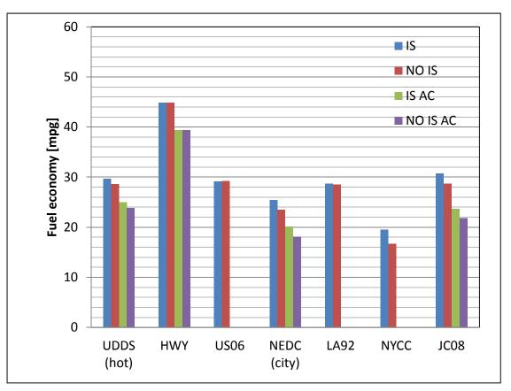
Figure 2. Mazda dynamometer test results comparison.
