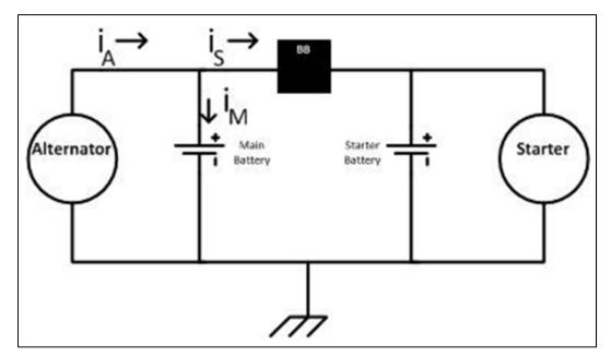
Figure 4. Mazda two-battery system schematic.
