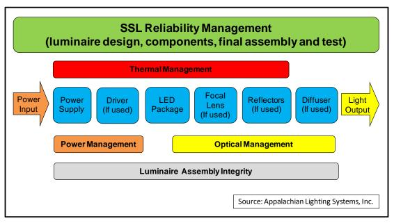
FIGURE 2. SSL LUMINAIRE COMPONENTS AND RELIABILITY CONSIDERATIONS SOURCE: APPALACHIAN LIGHTING SYSTEMS, INC.
