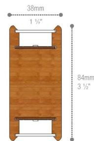
**Figure 3-58 Bamboo Pendant designed by Koerner Designs won the DOE Sustainable Manufacturing of Luminaires Prize in 2020. The key features of design include a biodegradable bamboo luminaire body and flaxseed printed circuit board along with an easy end of life (EOL) deconstruction design. [101]**
