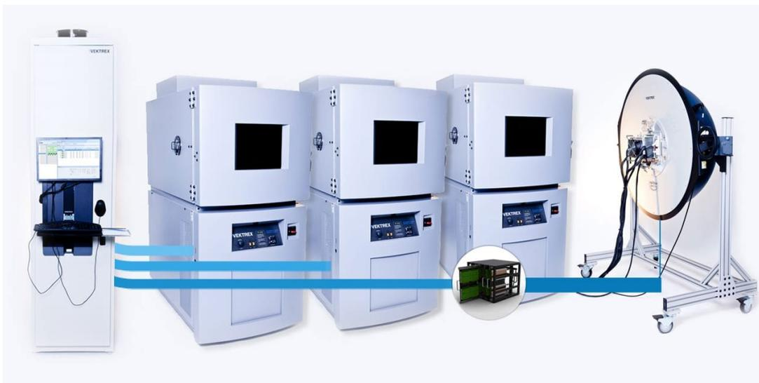
Figure 3-40 Reliability test equipment for LM-80 measurements. The LM-80 systems combine LED drive electronics with fully integrated thermal control systems and automated light measurement. [70]
