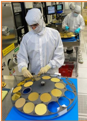
**Figure 3-13 Loading 150 mm wafers into a holder for an e-beam evaporator. [26]**
