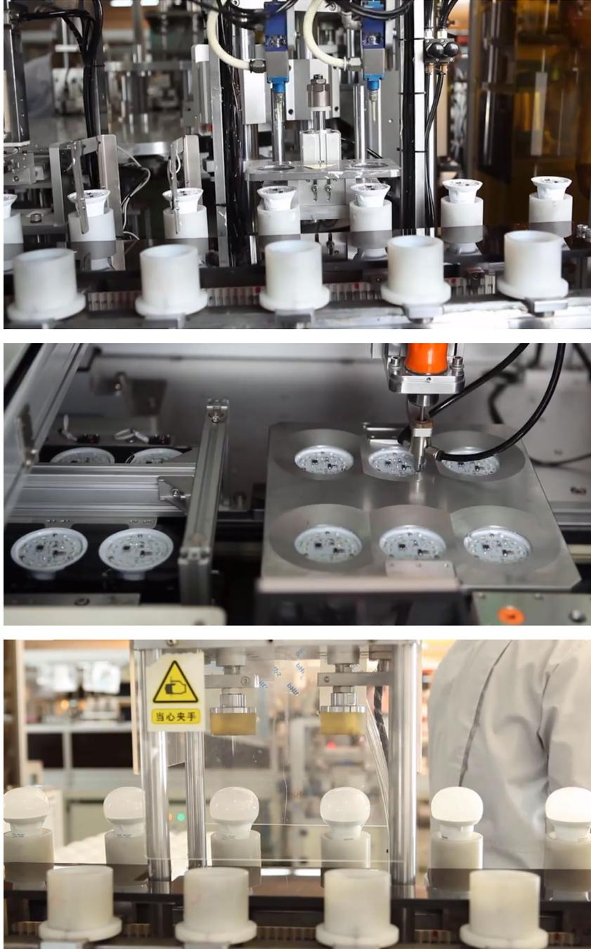
**Figure 3-48 Example of automated assembly lines for LED A-lamp. [81]**
