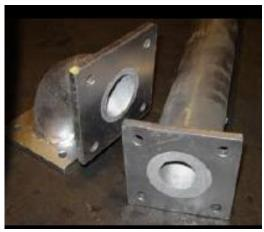
Pyrotek molten metal transfer piping
