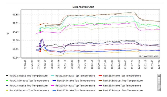
Figure 6 - Riptide Racks Intake and Exhaust Temperatures During Riptide Linpack Test
