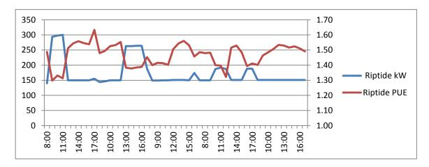
Figure 4 – Riptide PUE vs IT Load
