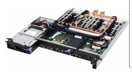
In 2011, the ASHRAE committee 9.9 published *Thermal Guidelines for Liquid Cooled Data Processing Environments*. This whitepaper introduced five environmental classes specifying operating temperatures and required cooling equipment for each class. Using the Direct Water Cooled iDataplex 360 M4 servers allows the MHPCC data center to run in ASHRAE liquid cool class W4.
