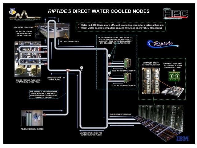
Figure 3 – Riptide's Direct Water Cooled Chips
