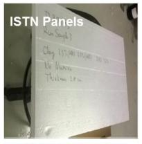
PS-clay composite foam board made in July factory trial. CO2/Ethanol blowing agent
