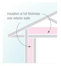
Raised heel or energy trusses allow even the corners of the attic to be well insulated; this helps to prevent ice dams in winter and keeps rooms cooler in summer.
