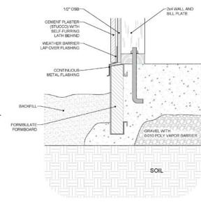
An ideal residential wall includes control layers providing rain, air, vapor and thermal barriers (based on Lstiburek 2009).
