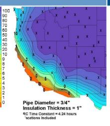
Integrated Collector Storage solar water heating systems are well suited to areas with little threat of freezing such as most of the California coast and southern Arizona. Other types of solar thermal water heaters are available including flat-plate collectors in indirect systems that use antifreeze; these systems work well in areas where freezing temperatures are possible. (Figure source: Jay Burch of NREL)
