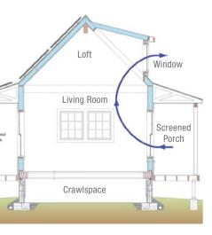
Building America's Building Science Consortium used convection to help cool this structural insulated panel (SIPs) cottage in Georgia. Cool air from the screened porches is drawn into the building's interior where it heats up and is pulled up and out the second-story windows, drawing more air in through the shaded first-story windows.
