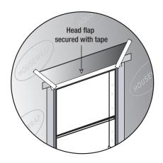
If headflap was created, fold it over the head flashing and tape across the top window flange and the 45° angle seams.
