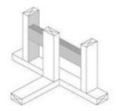
Ladder blocking where exterior walls intersect interior walls provides space for insulation and cuts back on thermal bridging.
