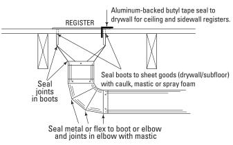
Mastic is a gooey adhesive that is applied wet. It fills gaps and dries to a soft solid. Mastics may or may not contain reinforcing fibers, and they may be used with reinforcing mesh tape.
