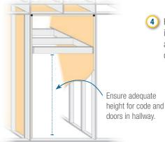
4 HVAC contractor installs sealed and insulated ducts in chase.
