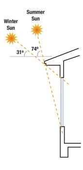
Sun angles for Albuquerque, NM. A 4-foot window would need an overhang extending 19 inches with 12 inches of wall above the window.
