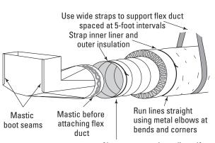
Never puncture inner liner. If repair is needed; install a coupling and seal properly
