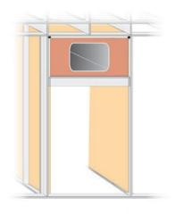
5 Drywallers finish exposed surfaces with sealed, caulked, taped, and mudded drywall and seal connection of duct boot to drywall.
