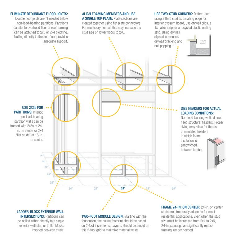
An example of a detailed wall framing layout. Use detailed layouts like this to make sure studs align from first floor to second floor to roof.
