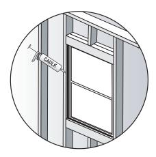
• On the interior side of the window, seal gap between the window and the rough opening with appropriate sealant.
