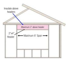
Using single 2x4 headers instead of double 2x6 headers in non-load-bearing walls allows space for insulation.
