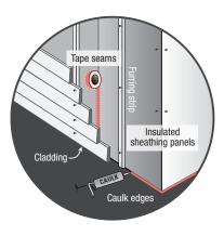
An exterior air barrier system, like rigid foam insulating sheathing, can provide a continuous air barrier when seams are taped or caulked. Furring strips attached over the foam allow the foam to act as a drainage plane and the space to serve as a ventilation gap, which is especially important under porous claddings like brick and stucco.
