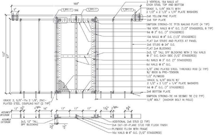
This advanced framing wall panel for seismic regions was designed and tested by Building Science Corporation and the U.S. Army Construction Engineering Research Laboratory (CERL) with funding by DOE's Building America program.
