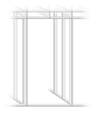
2 Install drywall or OSB or other air barrier extending past the area to be included in chase. Framers may install gypsum board.
