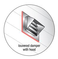
Dryer vent exhausts must have a gravity or other backdraft damper. A single hinged door with a 2½-inch effective opening is not as effective as a louvered damper.
