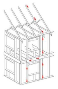
Advanced framing techniques include aligning wall studs with trusses and using single top plates.
