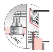
Provide bathroom and kitchen exhaust fans. Duct them to the outside and caulk ducts at the dry wall for an air-tight seal. Use low sone fans for quiet operation.
