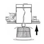
This LED fixture, the LR6 LED downlight by Cree LED Lighting Solutions, Inc, fits into a standard recessed can fixture and provides comparable light output to CFL and incandescent bulbs, at lower wattage and much longer life.
