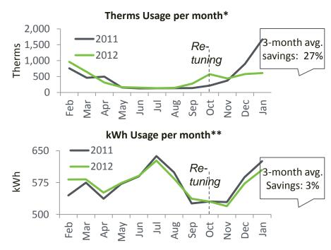
\*Both Therm and kWh usage were normalized by degree days \*\*Fan and cooling kWh savings are most significant during the Spring and Fall months
