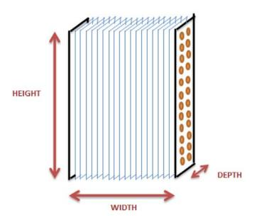
Figure 1: Evaporator Coil Dimensions
