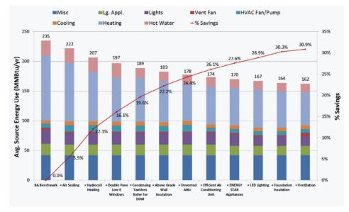
CARB used the National Renewable Energy Laboratory's BEopt energy simulation software to analyze each of the energy efficiency measures for optimized whole-building performance.
