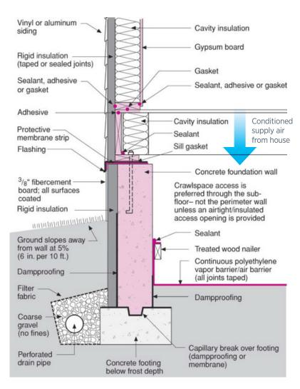
Insulating along the exterior wall is one option for an unvented crawlspace.
