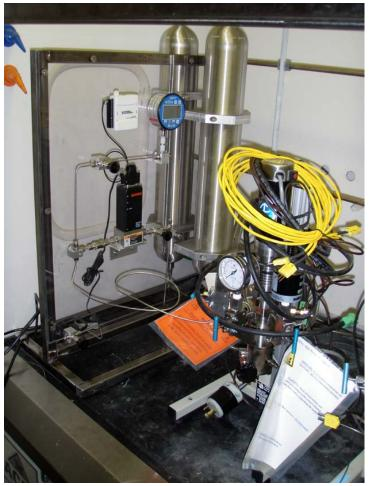
Reservoirs allow H<sub>2</sub> uptake measurement at constant pressure,
