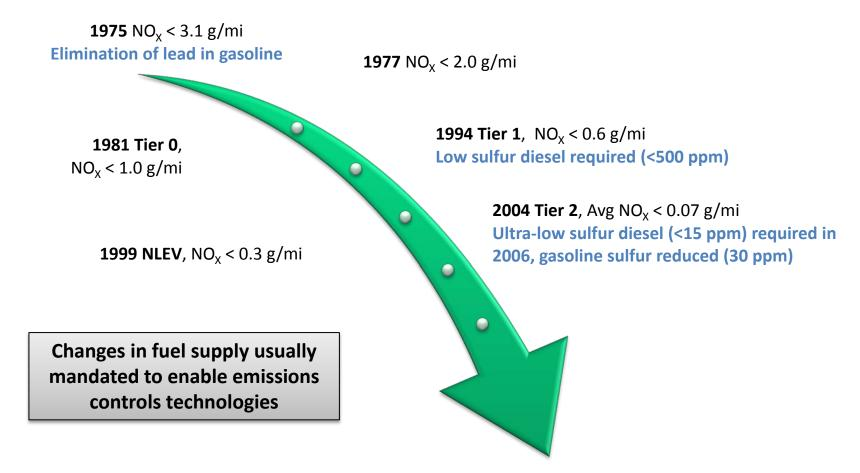
**2017 Tier 3**, Avg (NMOG + NO<sub>x</sub>) < 0.03 g/mi **Gasoline sulfur < 10 PPM, Ethanol in certification fuel**
