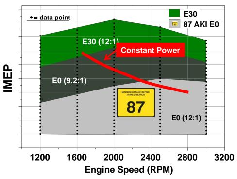
In a <u>high compression</u> research engine, highoctane E30 enables doubling of available torque compared to 87 AKI E0 fuel
