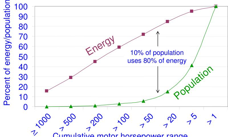
Cumulative motor horsepower range
