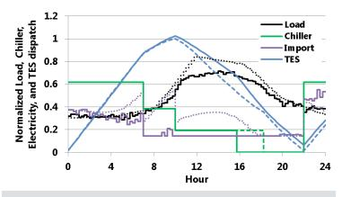
Example diurnal dispatch of chiller plant and thermal energy storage system using model-predictive control. *Results courtesy of University of California, Irvine.*
