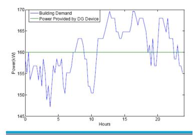
The dynamic nature and non-coincidence of building energy demands with power generated by distributed energy resources creates a challenge for system control and integration. *Illustration courtesy of University of California, Irvine.*
