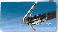
Hydrocarbons are "lifted" to the drillship by inducing nitrogen in the drill pipe. Rubber diaphragms minimize seawater ingress near the insertion tube inlet which significantly reduces the appearance of hydrates.
