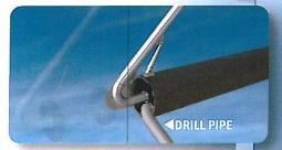
Rubber diaphragms conform around drill pipe to plug riser as much as possible.
