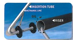
Insertion tube is guided into riser.
